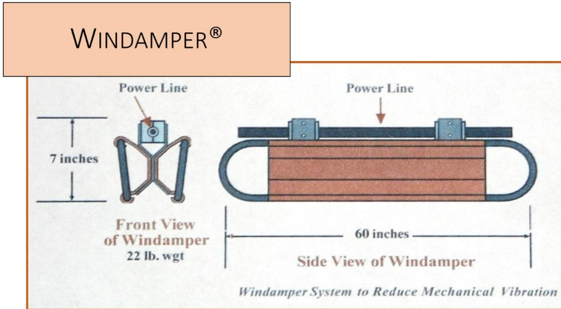
Each Windamper unit consists of two panel/bracket assemblies, two clamps and hardware. Field assembly necessary to join the two panel/brackets before attaching the clamps to the assembled damper during installation on the line. Armor Rods are required.
